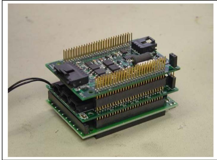
*Figure 3-1: RAS-500 Controller Stack*
