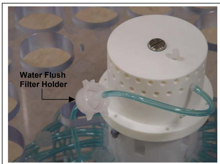
*Figure 5-2: Water Flush Filter Holder*
