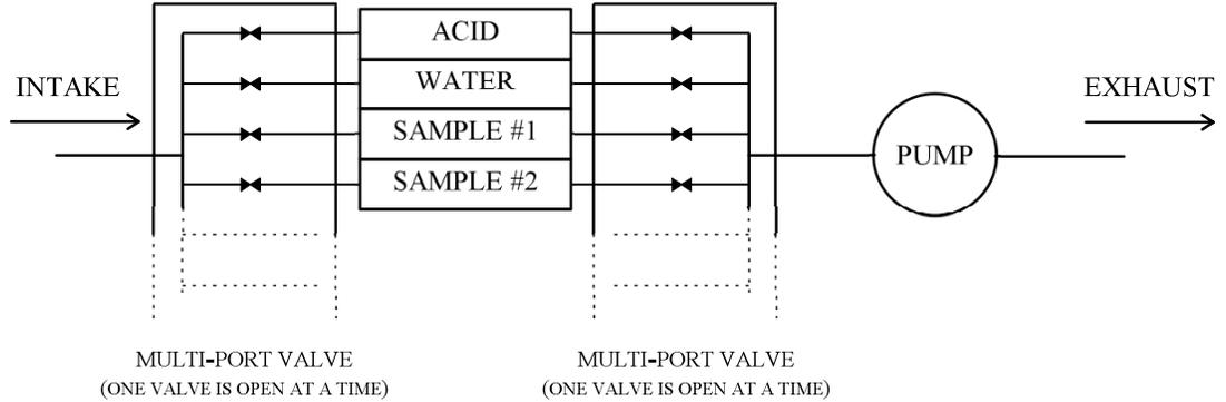
*Figure 2-13: Pumping Operation Schematic*
