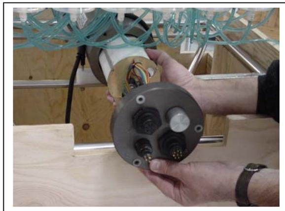
*Figure C-3: Remove Controller Housing through Notch in Stand*
