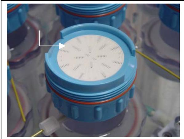
*Figure 5-4: Sample Tube with Filter Holder*
