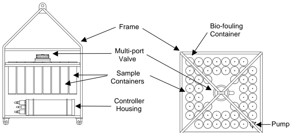
*Figure 1-1: RAS-500 Line Drawing – Overall View*
