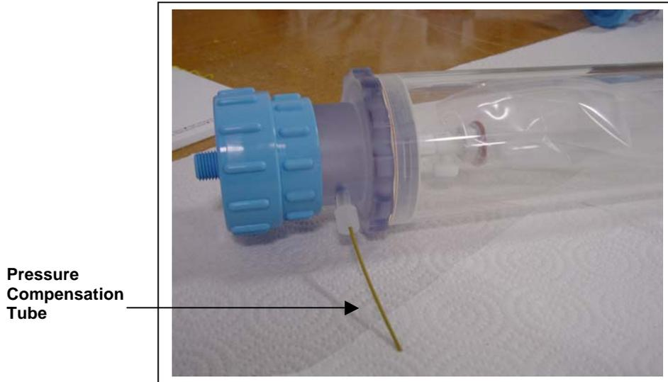
*Figure 2-6: Sample Tube with Luer Bag Installed*
