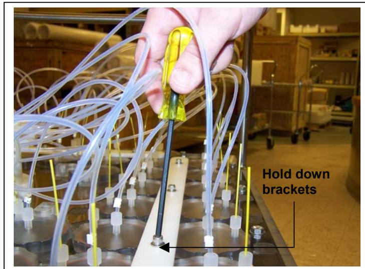
*Figure 5-6: Removing Hold Down Brackets*
