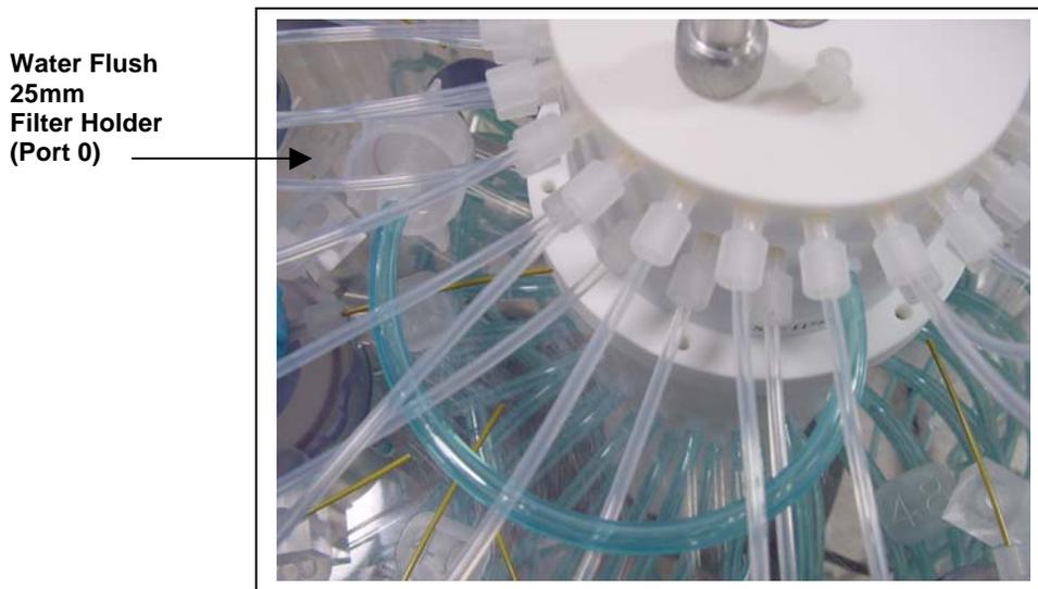
*Figure 2-14: Water Flush Filter Holder*
