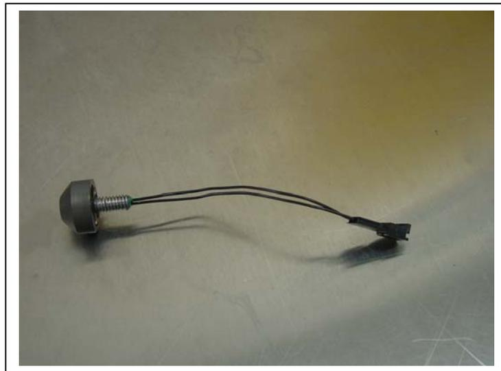
*Figure B-1: Thermistor External Temperature Sensor*
