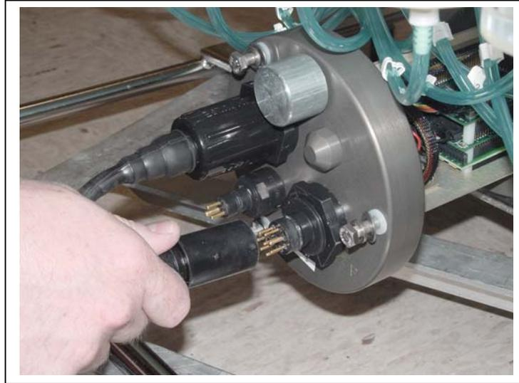
*Figure 2-5: Aligning Cable Connectors with Thumb Bump*
