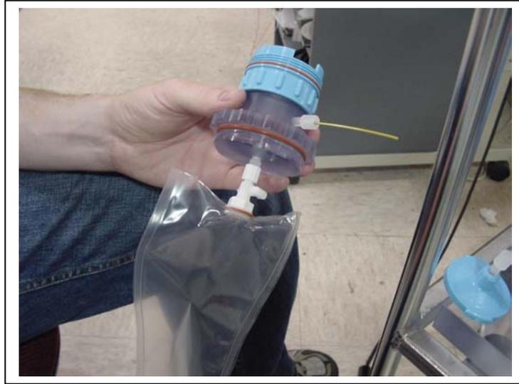
*Figure 5-11: Attaching a Sample Bag*
