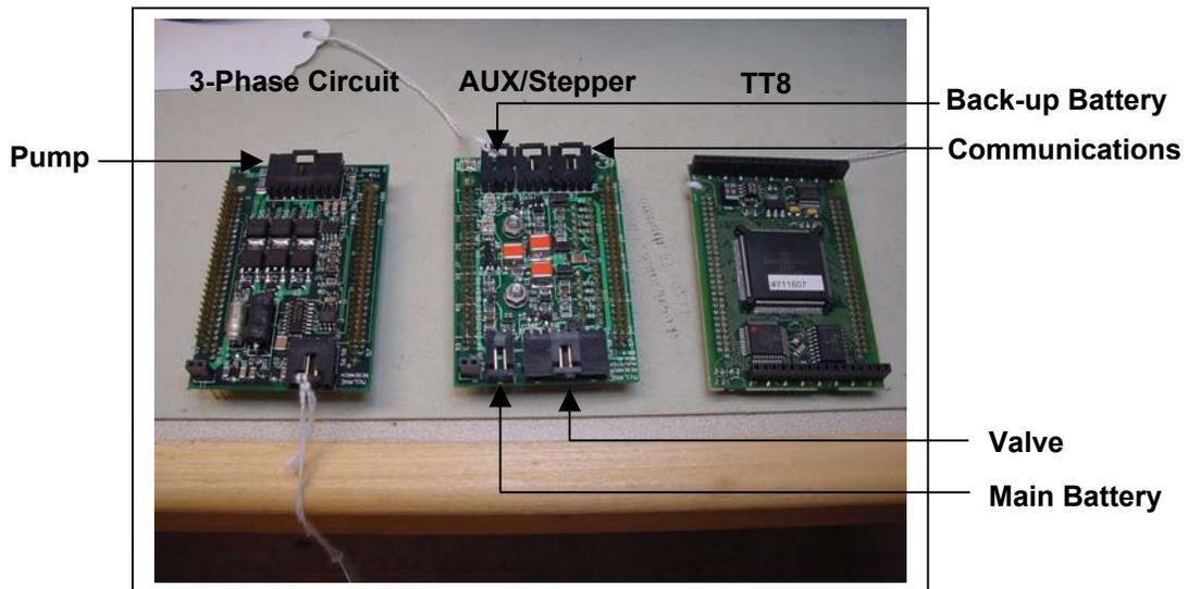
Figure 3-2: Three Boards of Electronics Stack
