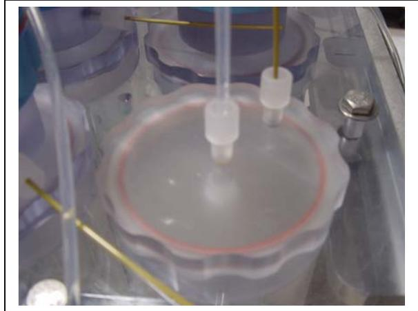
*Figure 5-5: Sample Tube without Filter Holder*
