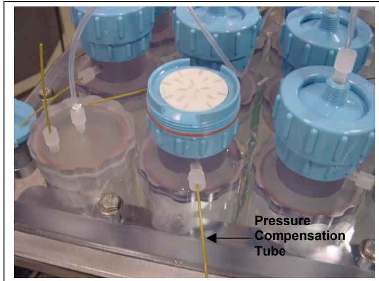
*Figure 5-7: Pressure Compensation Tube*
