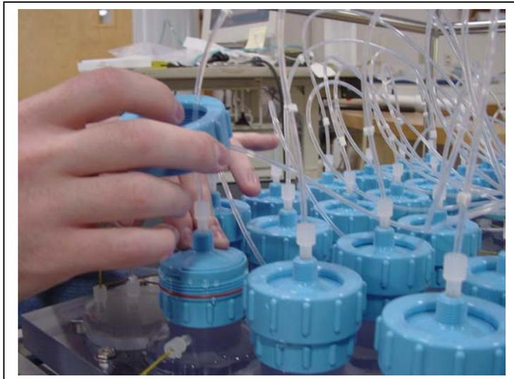
*Figure 5-13: Closing the Filter Holder Cap*
