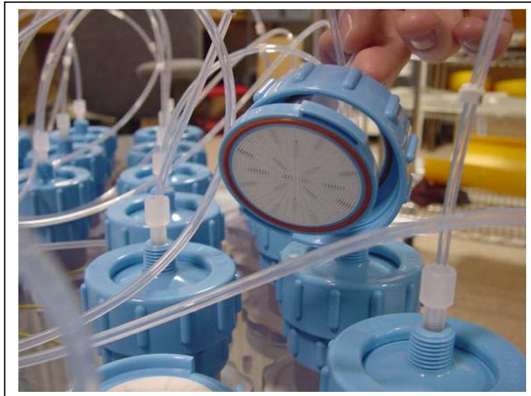
*Figure 5-8: Removing Filter Holder Tops*
