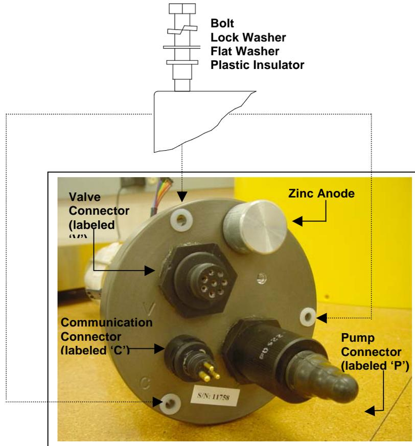
Figure 2-4: Controller Housing End Cap Bulkhead Connectors
