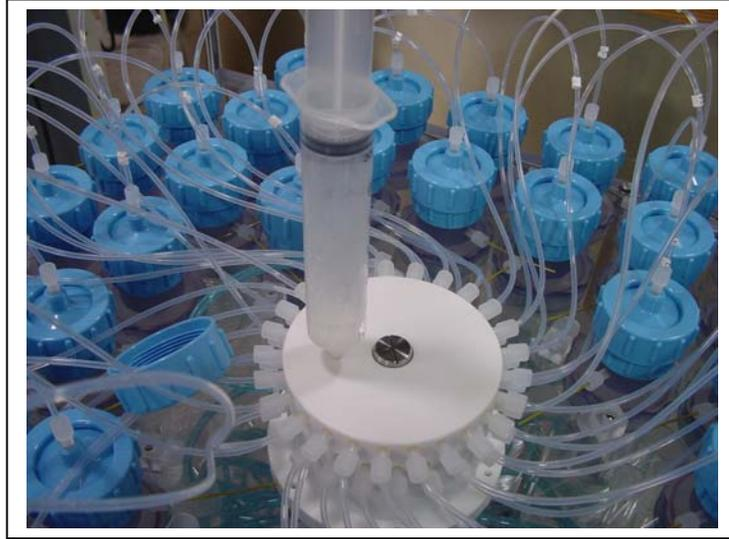
*Figure 5-12: Injecting Water into the Valve Intake*
